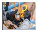
The RIG features a safety gate on the moving side plate that allows the rope to be installed easily while the device remains connected to the harness.
